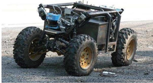
Figure 11.1 The Groundhog robot is a 1,500 pound custom-built vehicle equipped with onboard computing, laser range sensing, gas and sinkage sensors, and video recording equipment. The robot has been built to map abandoned mines.
