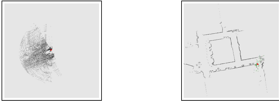
Figure 14.4 Mapping without odometry. Left: Raw data, right: map, generated on-line in real-time.
